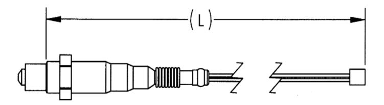
The sensor is still supplied with the universal crimp connector and insulating heat shrink tube and is pre treated with anti-seize compound.
