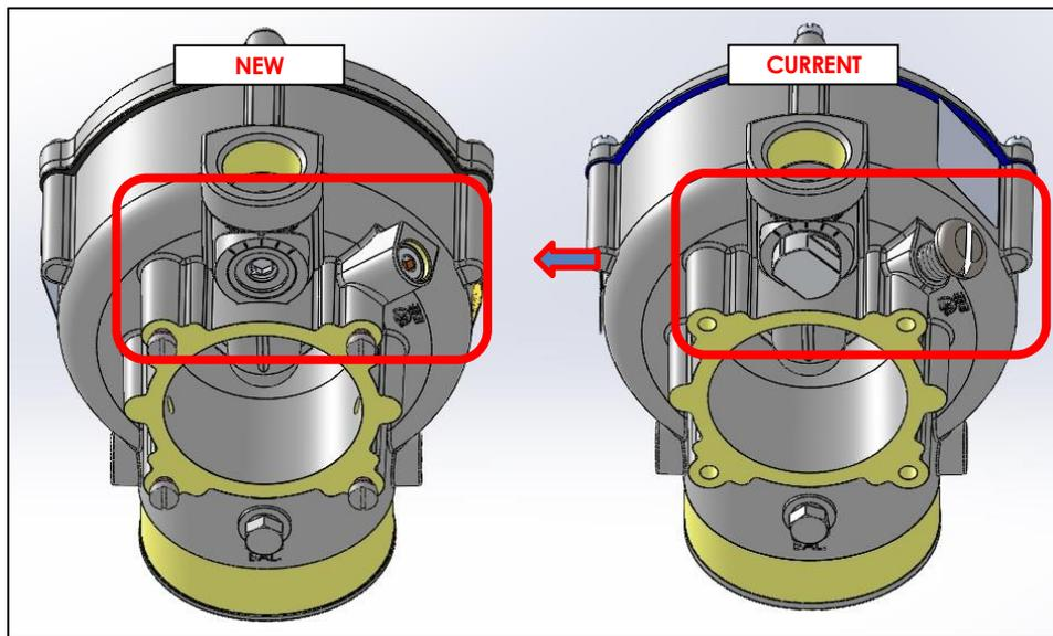
The new diaphragm cover will increase the overall height of the part by approximately 0.090" (2.3mm).
