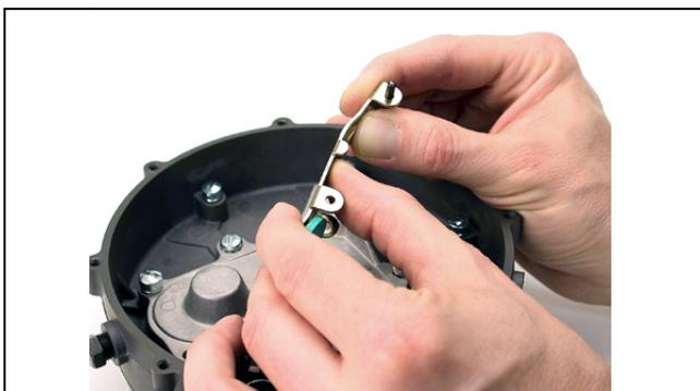
37. If necessary, remove the fulcrum pin (8) and lever (5) and bend slightly if required. Do not attempt to bend the lever when installed--unnecessary force on the lever may damage the secondary seat (6).
