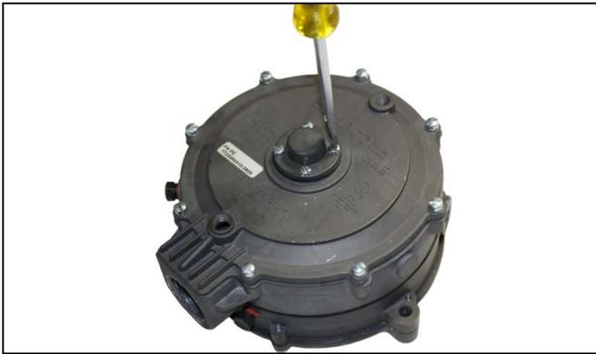
46. **PE Only** (Skip for E): Install the gasket (28) and spring housing (27). Align the spring retainer housing screw holes to the cover (26) and insert cover screws (23). Torque to 7-11 in-lbs.(0.8-1.2 Nm).
