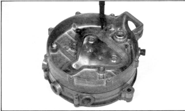
26. Install the primary diaphragm (13) over the locating pins and screw bosses, providing alignment for the assembly of the springs (12) and cover (11).
