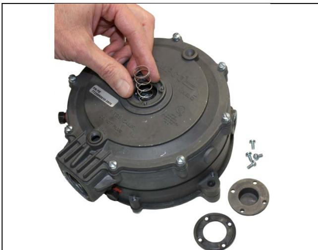
2. **Model PE Only** (Skip for E): Remove the spring retainer housing cover screws (27) and cover (28). Remove the housing gasket (29) and secondary spring (7).
