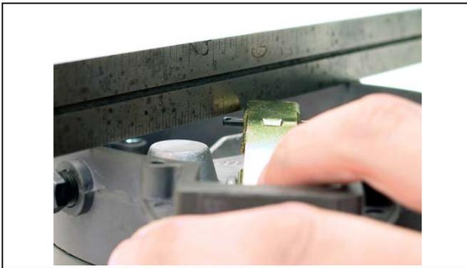
36. Lightly pull the lever (5) up against the secondary seat for measuring. Use a straight edge or the IMPCO G2-2 gauge to check the lever height. The secondary lever link pin should be approximately  $1/32$ " (0.8mm) below the level of the body casting. If the lever height is incorrect, continue to Step 37. Once the lever height is correct, skip to Step 38.
