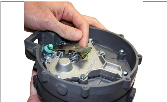
40. **Model E Only** (Skip for PE): Slip the spring (7) under the secondary lever (5) making sure it is retained by the two tabs at the sides and the single tab punched through the top of the lever.
