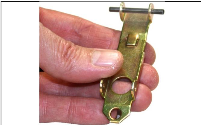
31. Inspect the tabs on the lever (5) to verify they are not bent and the pin (26) is centered.
