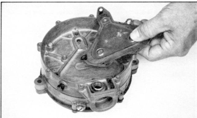
25. The new primary diaphragm assembly (13) is ready to be put into place.
