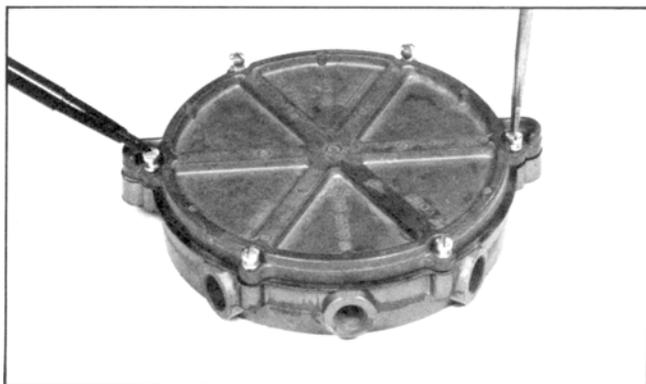
20. Reassemble the back cover (22) and gasket (21) to the heat exchanger body (19). Replace six screws (2). Match the mounting bosses in the cover with those on the heat exchanger. Tighten the two screws shown in the photo first, then upper and lower screws diagonally opposite to draw the cover down evenly. Torque to 25-35 in-lbs (2.8-4.0 Nm).
