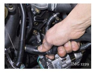
38. Remove old regulator coolant hoses and connect the new IMPCO regulator hoses and tighten the clamps. NOTE: Coolant hoses are intentionally 6" long. To prevent kinks, cut the hoses to the correct length if necessary.
