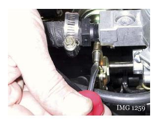
51. Adjust the vacuum dashpot adjustment screw to 800 RPM at tilt relief with the transmission in neutral.
