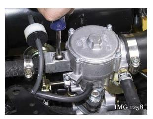
54. Set the power adjustment on the carburetor. With the wheels blocked, parking brake on and foot on the brake pedal, depress the accelerator to full throttle position with the transmission in drive. Set the CO to 0.80%. \*
