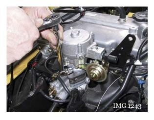
17. Install the IMPCO carburetor to the adapter plate using a new gasket, nuts and washers provided. Tighten the nuts evenly to 17 lb ft (23 N•m).
