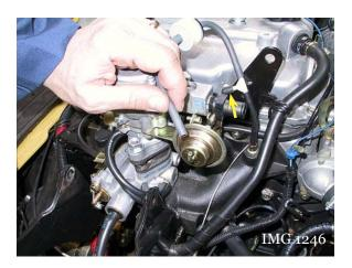
19. Remove the loose vacuum hose from the tee fitting and cap with the vacuum cap provided. Connect the end of the remaining vacuum hose to the carburetor vacuum dashpot.
