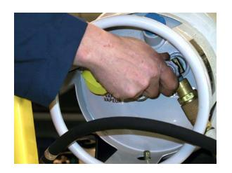
48. Open the fuel tank supply valve and perform a leak check at all fuel line and vapor hose connections. Repair leaks if necessary.
