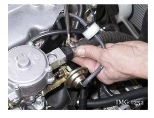
42. Connect the fuel vapor hose from the regulator to the carburetor and tighten clamp.
