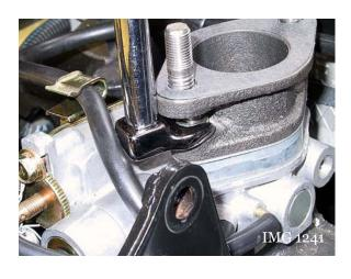
16. Install the IMPCO carburetor adapter using a new gasket provided. Use the previously saved nuts and washers. Tighten the nuts to 17 lb ft (23 N•m).
