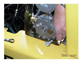
37. Install the new IMPCO regulator/lockoff assembly to the same location as the old regulator. Be sure to re-attach the electrical ground strap to the bracket. Tighten the regulator assembly bracket bolts to 17 lb. ft.  $(23 \text{ N} \cdot \text{m})$ .
