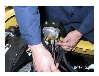
39. Connect the fuel tank high pressure hose to the vacuum lockoff inlet fitting. Torque fitting to 20 lb. ft. (27 N•m).
