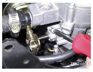
52. Adjust the engine idle speed at the carburetor to 800 RPM in neutral.
