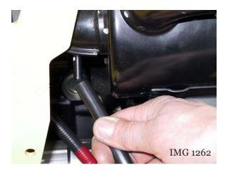
46. Reinstall the governor vent hose to the air cleaner housing.
