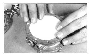
29. Press Filter (13) so that's properly seated in recess.
