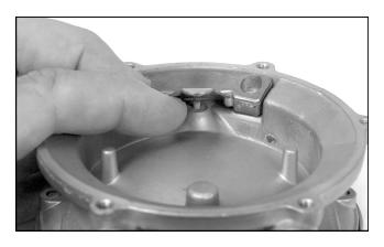
34. Lift Lever (6) to ensure it moves properly and verify that the Valve Pin (10) follows lever travel.
