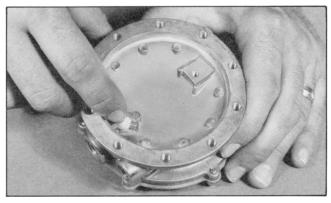
24. Place the Seat (19) with the viton (black rubber) side down, in position on jet.
