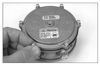
36. Place Cover (2) in correct position and insert Screws (1).
