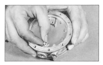
21. Lubricate the Pin Valve (10) with petroleum jelly and insert through hole in the Washer Retainer Seal (14) and Lip Pin Seal (9). Rotate head of Pin gently in a circular motion to ease Pin into place through the Washer, Lip Pin Seal and Body (7) housing.
