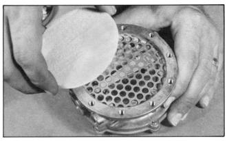
28. Insert Screen (12) and Filter (13) into recess.
