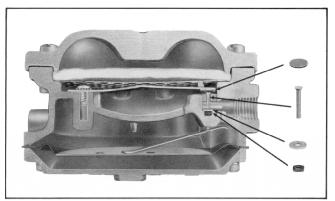
9. Cutaway shows assembly of Valve Spring (11), Valve Seat (19), Valve Operating Pin (10), Seal Retaining Washer (14) and Pin Lip Seal (9). Note that removal of Valve Pin allows retaining Washer to be removed through the ½" NPT opening labeled "Out."
