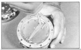
26. Replace Spring (11) and fasten in place with Screw (4). Align the tip of Spring (over valve) and center between the 3 guide fins as shown in illustration. Tighten Screw 28-32 in-lbs. (3.2-3.6 Nm)
