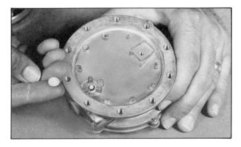
23. Valve Seat (19) shown with aluminum side up ready to be placed on jet.
