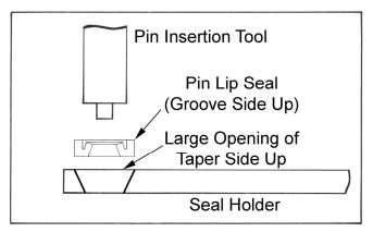
15. Lubricate the Lip Pin Seal (9) with petroleum jelly or Vaseline and place in the Seal Holder Insertion Tool groove side up, as shown in the illustration. Note that the Seal Holder passage is tapered and the wide opening of the seal holder should be facing up.
