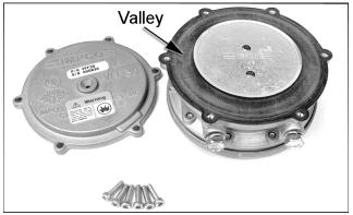
35. Turn Diaphragm (3) so the gasket side is down (see illustration on page 2) place on the Body (7) and rotate to position so the screw hole pattern aligns with the holes in the Body (there is only one position in which the holes will line up).
