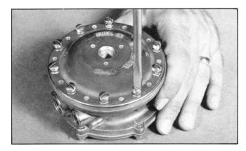
33. Tighten Screws (17), alternating from side to side on opposite sides of the cover until all screws are solidly set. Torque to 60-70 in-lbs. (6.8-7.9 Nm).
