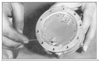
11. Using the same hook, remove the Pin Seal (9) through valve jet.
