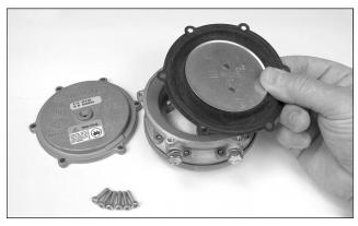
13. Remove Cover (2) and diaphragm (3). Clean covers, body and metal parts as necessary with a safety solvent and dry prior to reassembly.
