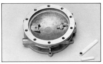
16. Place the VFF30 Body (7) with the filter side up, as shown in the photo, on a flat surface. Ensure that the groove in the Seal (9) is visible from the top of the taper of the Seal Holder Insertion Tool.
