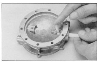
18. Coat the Pin Insertion Tool with petroleum jelly and push the Seal (9) through the Holder and into the Seal recess of the VFF30 Body (7). Look through the fuel port to ensure the Seal is seated in the seal recess and that the groove in the seal is visible.
