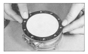
30. Place Gasket (15) in place and align with screw holes.
