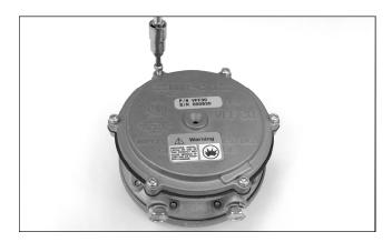
12. Remove 6 Screws (1) on diaphragm cover side.
