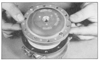
31. Insert two Screws (17) opposite each other in the "Fuel In" cover and place on Gasket (15). Thread the two Screws (17) through the gasket and into the Body (9).
