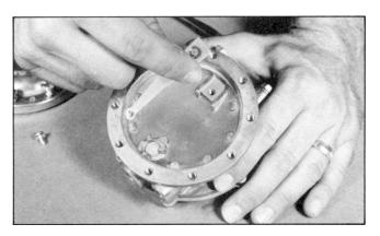
25. Spring (11) ready to be fastened in place. Be sure the arc in the center faces upward (see illustration in step 26 below).
