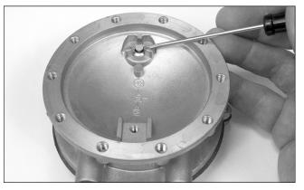
7. Gently lift up and remove the Valve Operating Pin (10).
