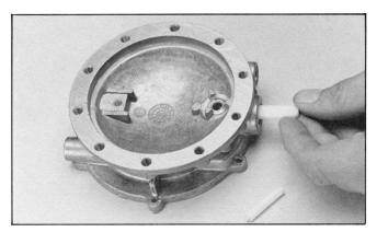
17. Place the holder in the up position and slide the Holder and the Seal (9) into the Body (7) of the VFF30. Looking through the fuel port, position the Seal above the cavity of the seal recess.
