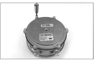
37. Tighten Screws (1) alternatively from side to side across cover until all are solidly fastened. Torque to 28-32 in-lbs. (3.2-3.6 Nm)
