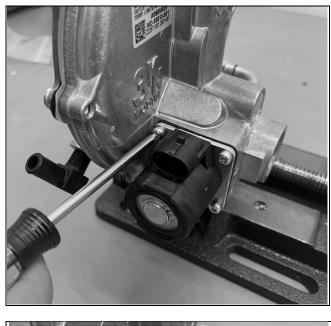
Using a T20 Torx screwdriver, remove the four (4) 8-32 TORX SCREWS holding the lock-off valve to the regulator.
