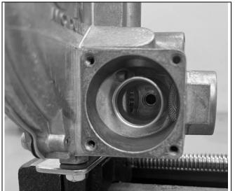
Inspect lock-off bore and screw taps for any residual debris or material; if present, carefully remove with tweezers or pick. DO NOT spray with compressed shop air to remove.
