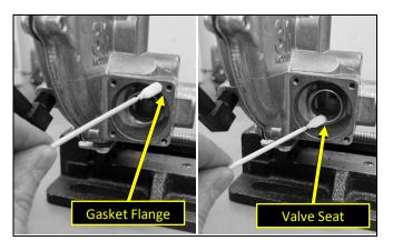
Using a lint-free Q-Tip and isopropyl alcohol, thoroughly clean both the gasket flange and the lock-of valve seat surfaces of the regulator body. Inspect both surfaces for chips or dents that would affect sealing – if any are identified, the complete regulator will need to be replaced.
