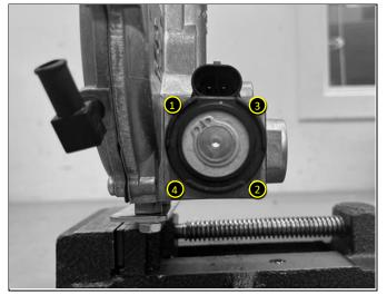
12. Straighten the GASKET to properly align the GASKET screw holes with the regulator body flange screw holes. Hand-start the remaining (3) 8-32 TORX SCREWS into the screw holes in the regulator body.
