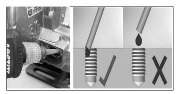
5. Add Loc-Tite 242 or approved alternative to the lock-off flange bolt hole threads. DO NOT get Loc-Tite anywhere else on the flange.
