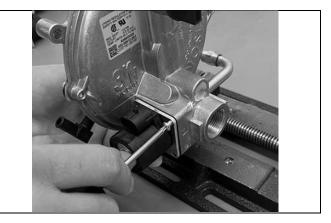
Use a lint-free Q-Tip to apply a thin layer of Xiameter PMX-200 silicone fluid (or equivalent) to the sealing surface of the PLUNGER ASSEMBLY
