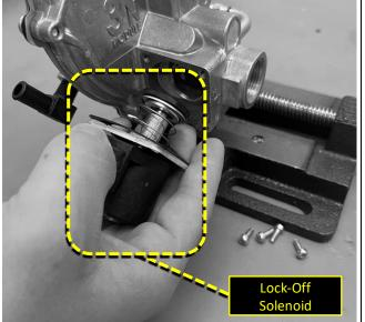
2. Remove all LOCK-OFF SOLENOID components from the regulator, as well as the sealing gasket.
